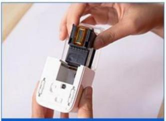
3. Put the ink cartridge into the ink tank of the printer.
